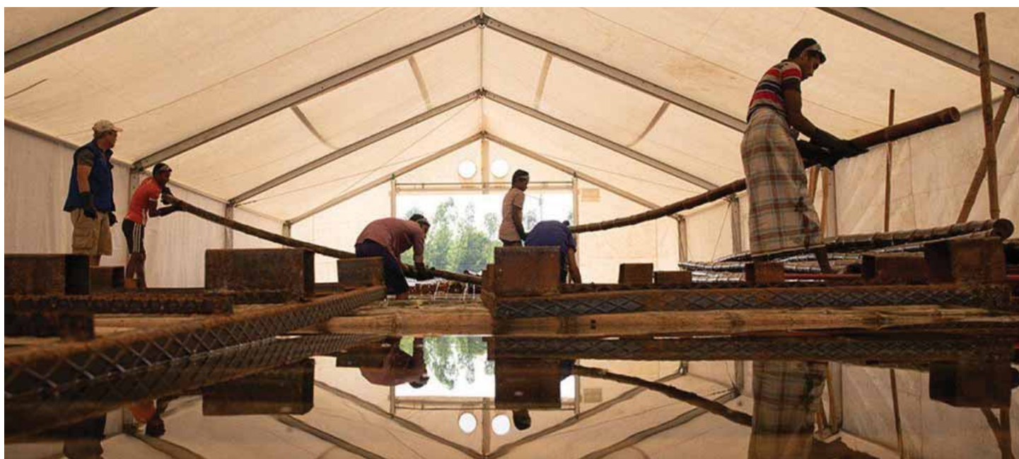
BAMBOO TREATMENT PLANT PROVIDES SHELTER TEAM WITH BEETLE RESISTANT BAMBOO © IOM 2018
